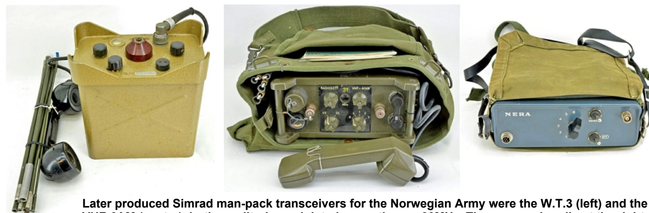
Developed and produced by Simonsen's 'Simrad' was the W.T.2, a miniature man-pack set with 5 channels operating around 30MHz. On the photo in the centre is Willy Simonsen testing a W.T.2.
